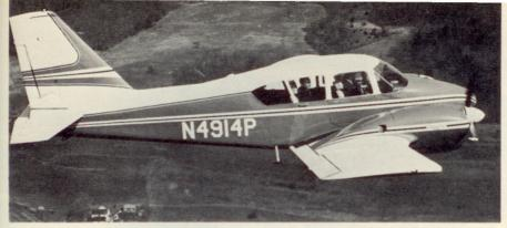
New Piper Apache 235 is reported by manufacturer to combine speed, utility and short-field ability with economy. It is distinguished by long, sleek hull, swept tail and single-piece stabilator
